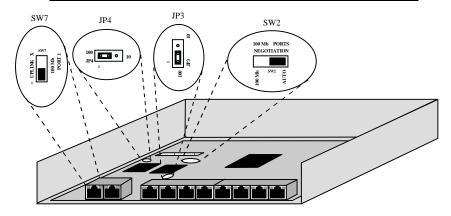
Figure 3.5: Magnum 528's internal jumpers for auto-negotiation ON or OFF
